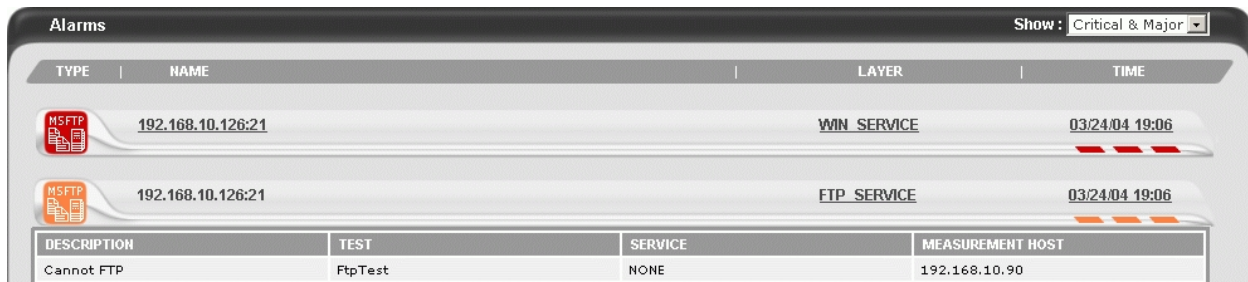
Figure 1.9: A Major alarm indicating that the agent is unable to FTP files
