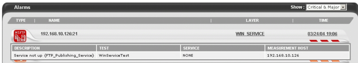
Figure 1.8: The Critical alarm indicating the MS FTP service has gone down
